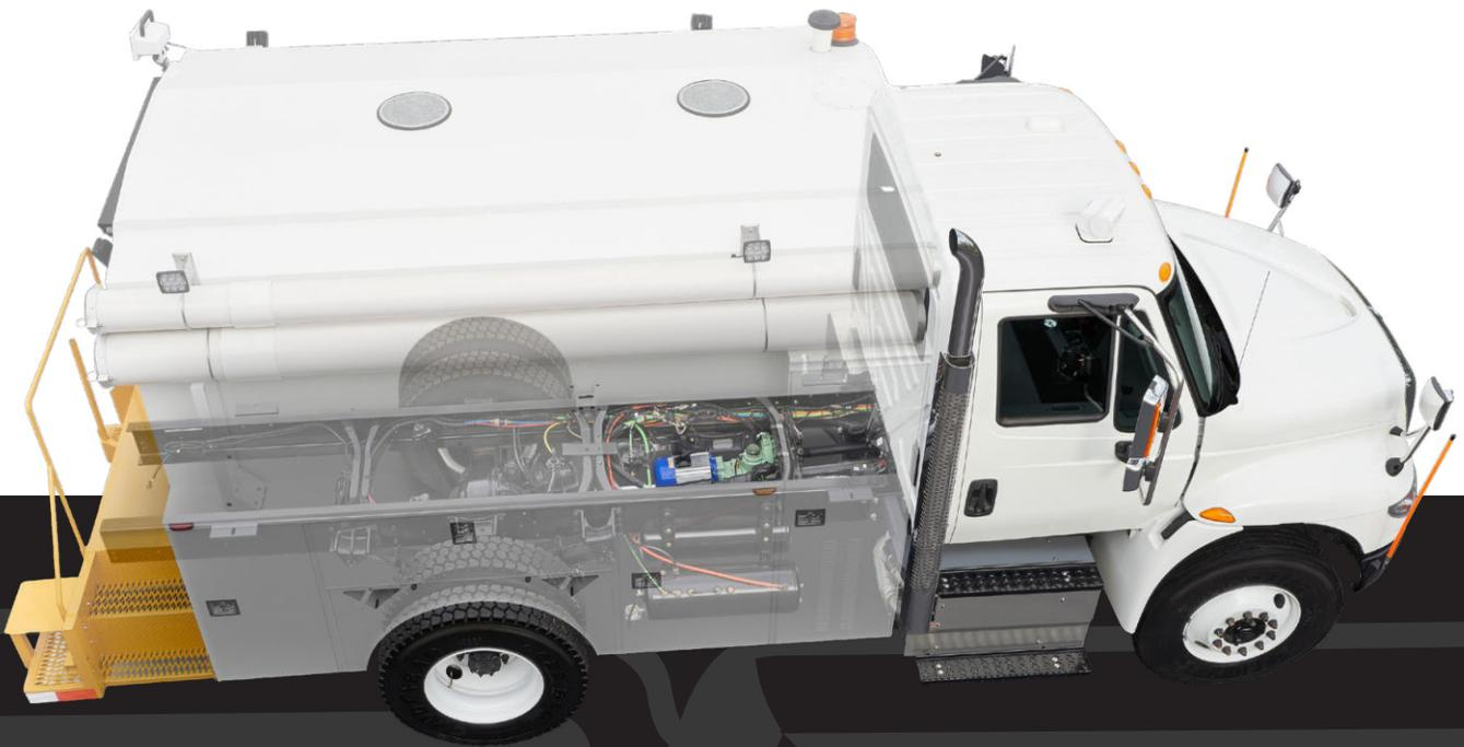
Utilizing the vehicles own engine for power, Vanair® underdeck rotary screw compressor systems provide you with the exceptional power your crew needs to get the job done where and when they need it. Using a single PTO opening and mounted seamlessly out of sight, under the vehicle, these systems provide up to 300 CFM\* of impressive air power, AC power or hydraulics, or any combination of all three.
