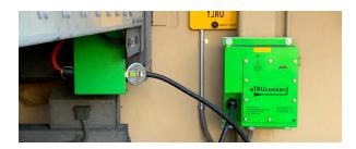
Unlike competing technologies, ESL's innovative design does not require 2 extra pilot pins at the connector. A connection detection device is embedded in the safety-interlocked IEC female plug installed at the end of the cable. This allows truck owners to use the OEM provided inlet for plug-at-front configuration or retrofit their fleet with ESL's cost effective plug-at-rear kit.
